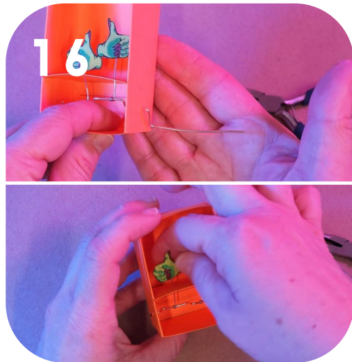
16 Bend crank shaft tail into a crank. Straighten hand rods, if needed.
